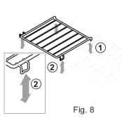
The **Flat Half Rack** has a removable insert that can provide extra space for larger food items. The right half rack portion may still be used for other food items like a casserole dish (See Fig. 5). To remove the insert, squeeze on the left front insert side (See Fig. 7) of the rack and tilt out clockwise. To reinstall insert rear hooks at back of insert (See 1-Fig. 8) and lay insert down. Make sure both insert front hooks snap into rack (See 2-Fig. 8).
